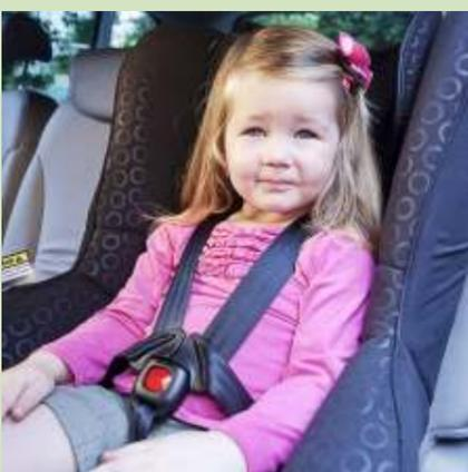
Forward facing combination child restraint with inbuilt six-point harness
